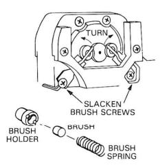
Cleaning of the commutator can be carried out by removing the brushes. This allows room for a paint brush, dipped in methylated spirit or lighter fuel, to be inserted gently. It will be found that by turning the wheels of the locomotive slowly a new area of commutator face can be brought into view, which may be cleaned in this way.
